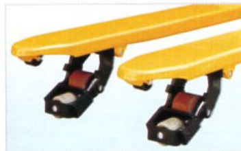
Additional wheels for sideways movement
